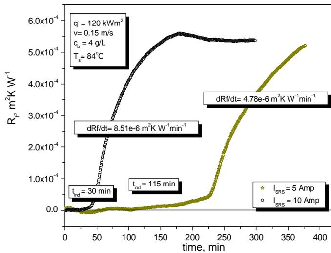
Fig. 14 Fouling resistance as a function of time of 1.55  $\mu m$  roughened stainless steel surfaces at 5 and 10 Amp
