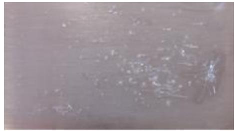
$R_a = 1.05 \mu\text{m}$ ,  $T_s = 75^\circ\text{C}$
