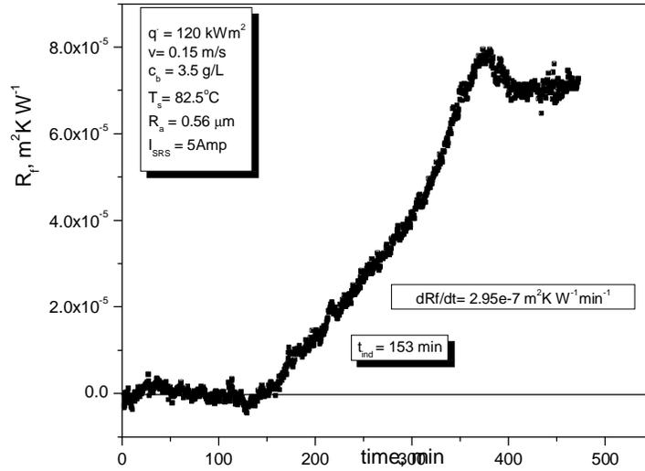
Fig. 8 Variation of fouling resistance with time as a function of SRS system of 0.54  $\mu\text{m}$  roughened surface
