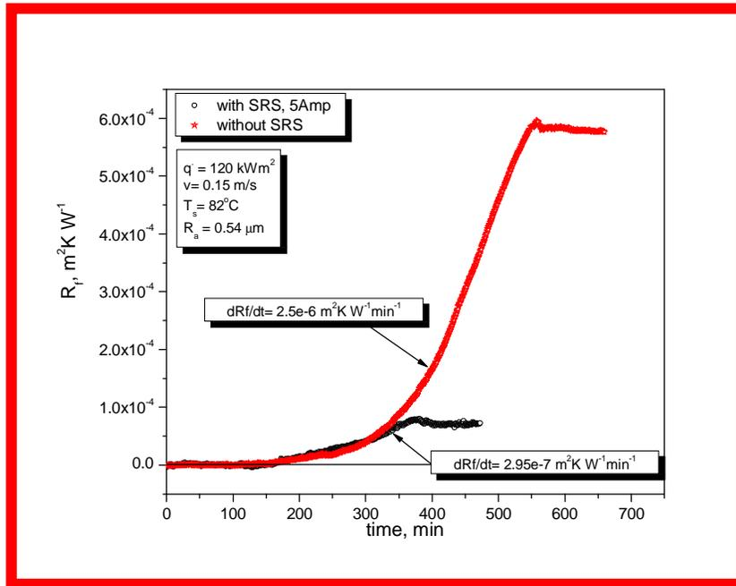
Fig. 10 Fouling resistance as a function of time of 0.54  $\mu\text{m}$  roughened stainless steel surfaces with and without SRS
