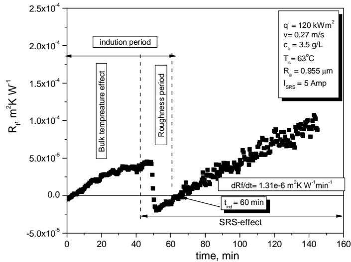
Fig. 2 Variation of fouling resistance with time as a function of SRS system of 0.955  $\mu\text{m}$  roughened surface
