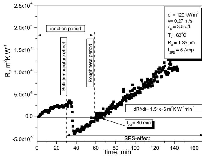
Fig. 3 Variation of fouling resistance with time as a function of SRS system of 1.35  $\mu\text{m}$  roughened surface
