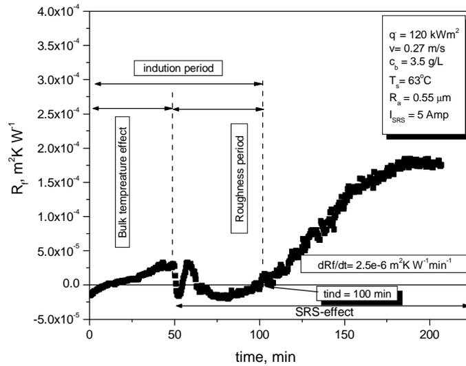
Fig. 1 Variation of fouling resistance with time as a function of SRS system of 0.55  $\mu\text{m}$  roughened surface
