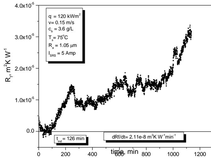
Fig. 9 Variation of fouling resistance with time as a function of SRS system of 1.1  $\mu\text{m}$  roughened surface
