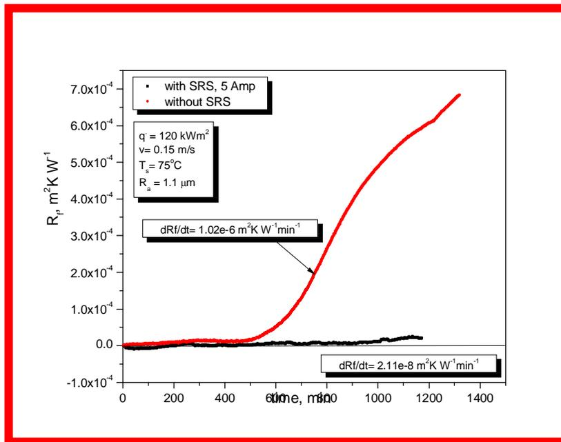
Fig. 11 Fouling resistance as a function of time of 1.1  $\mu\text{m}$  roughened stainless steel surfaces with and without SRS
