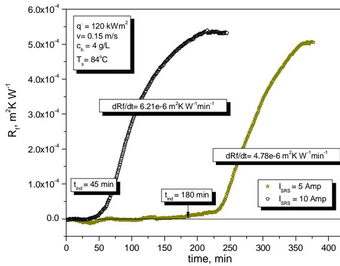
Fig. 13 Fouling resistance as a function of time of 0.54  $\mu m$  roughened stainless steel surfaces at 5 and 10 Amp
