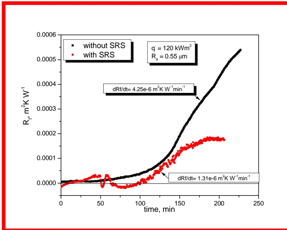
Fig. 6 Fouling resistance as a function of time of  $0.54 \mu\text{m}$  roughened stainless steel surfaces with and without SRS
